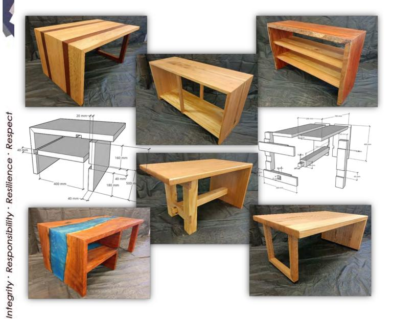
Year 11 Design & Technology students have consolidated their learning using Computer Aided Design (CAD), developing project drawings for production in the workshop. The task was to design and then construct a waterfall end coffee table, using a minimum of three timber joints in the construction.
